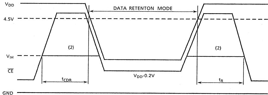
Note (2) : If the  $V_{IH}$  of  $\overline{CE}$  is 2.4V in operation,  $I_{DD2}$  current flows during the period that the  $V_{DD}$  voltage is going down from 4.5V to 2.6V
