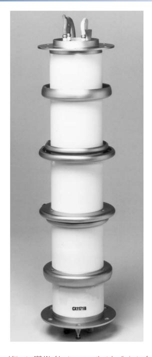
In addition to 400 W of heater power, the tube dissipates from 100 W per ampere average anode current, rising to 300 W/A at the highest rates of rise and fall of anode current. Both ends of the tube must be cooled whenever heater voltages are applied, since the cathode flange will reach a temperature of 120  $^{\circ}\text{C}$  above ambient in the absence of cooling. Envelope temperature:
