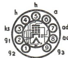
The BRIMAR UBF89 is a double diode vari-mu pentode. The pentode section is designed primarily for use as an R.F. or I.F. amplifier, and the diodes for A.M. detection.
