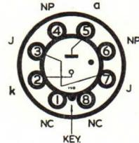
The VR75/30 is a cold-cathode, gas-filled, voltage-stabiliser for use in industrial and radio equipment where a stable source of voltage is required. It is equivalent to the U.S.A. OA3 type.
