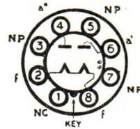
The BRIMAR type 5R4GY is a directly heated full wave rectifier for use in A.C. mains equipment where a large output is required.
